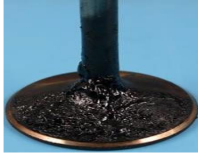
Intake Valve Deposits
